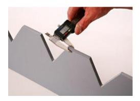
Utilizing suitable resin systems such as Vinyl Ester, Epoxy, Atlac etc. GRP composite plate can be manufactured to resist highly toxic and acidic chemicals. They make ideal GRP weir plates and scum boards which are generally offered at 6mm – 12mm thick and can be supplied pre-curved or as flat sheet to a max length of 3000mm. These boards are widely used in the water industry due to their versatility, low maintenance and easy of fit.
